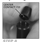
Place the CENTER CONTACT (12) on the TOOL (20) making sure the pins of the TOOL (20) are in the holes of the LOWER INSULATOR (13).
